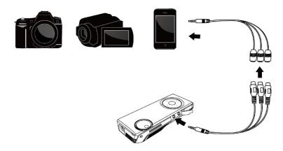
Some video devices do not have the standard audio and video connections and may require an AV cable specified by the vendor. The AV cable allows you to connect your video device to your TV monitor or your projector. Also may be purchased from the video device vendor. When you have the AV cable, use the cable adapter to connect the video device cable and The RMP-8200 CINEMA ON-THE-GO cable.
